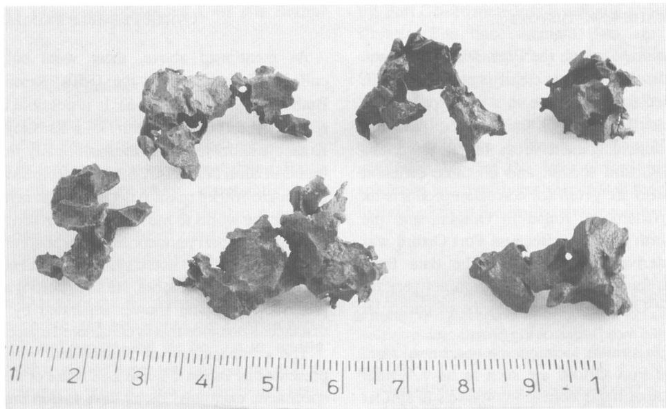
FIGURE 2-11.—Imilac (Copenhagen). Six fragments of the shower weighing 5-15 g each, collected on the site in the Atacama Desert, Chile, by V.F. Buchwald in 1973 (Buchwald, 1975:1395). The Port Orford specimen is similar to these but with better-preserved fusion crust and less deformation. Scale in cm.
