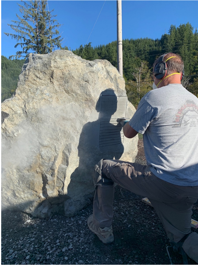
(L) Stu Richardson, Richardson Masonry, Reedsport, Oregon, cutting patterns into Umpqua Memorial Stone with diamond grinding wheel to house bronze plaque. (R) Stu chiseling sections from stone made by grinding wheel. Photos by Richardson Masonry apprentice, Jason Richer, October 15, 2023.
