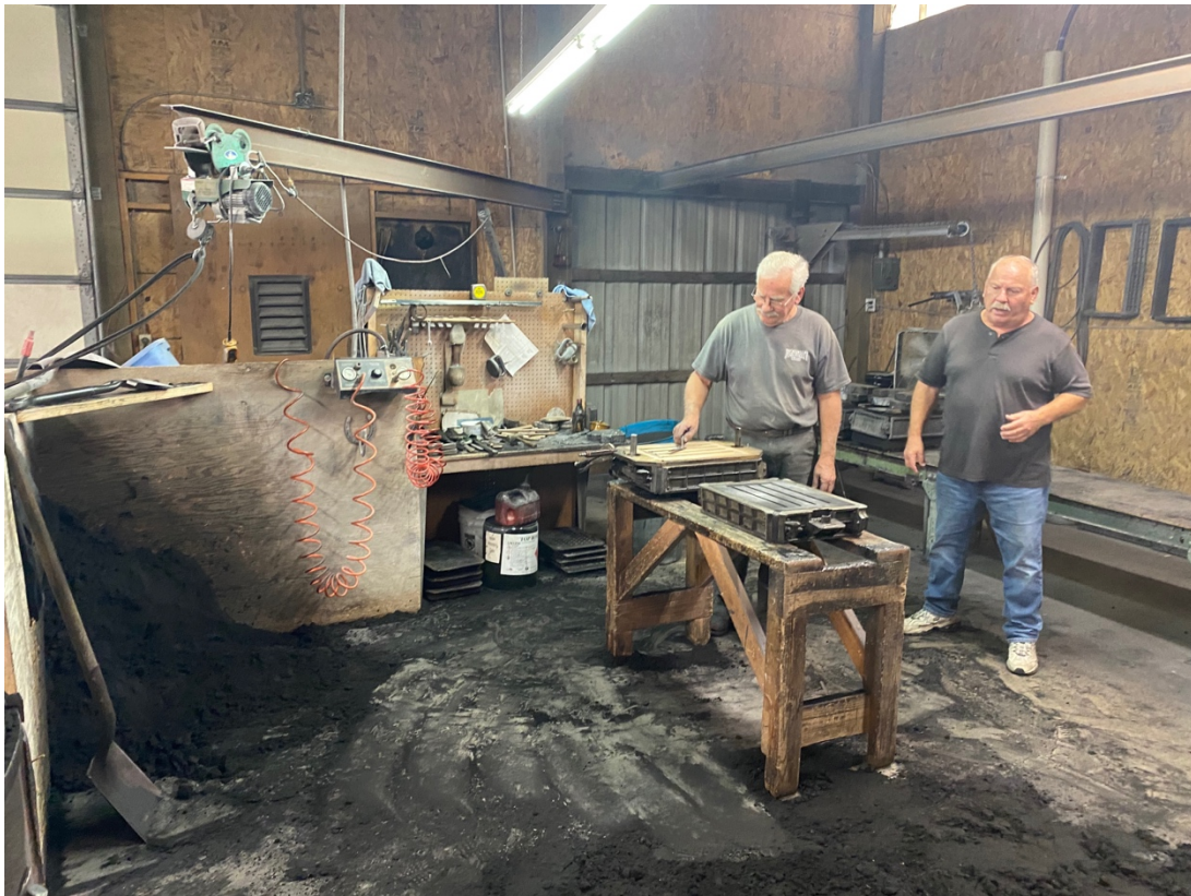
Phil Hager and father Larry at Bronzecraft Memorials, Wamic, Oregon. Phil has nearly 50 years' experience making molds and castings and "no one is better." The black sand across the floor was originally green and soaked with water before being impressed by the polymer template. It turns black from the heat of the melted bronze, which is poured onto the mold at 2300 to 2400 degrees F.
