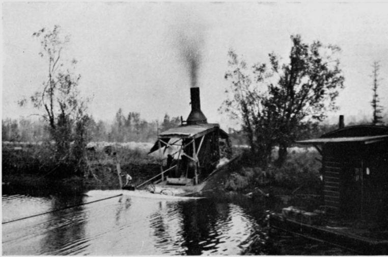
12 x 14 inch Humboldt Yarder about to ford a slough 160 feet wide, 8 feet deep, 150 pounds steam pressure.
