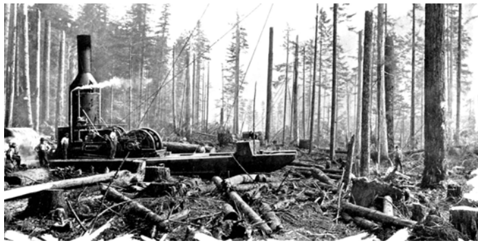
Willamette 11 by 13 steam donkey working in the woods. Photo is from the 1925 Willamette catalog.
