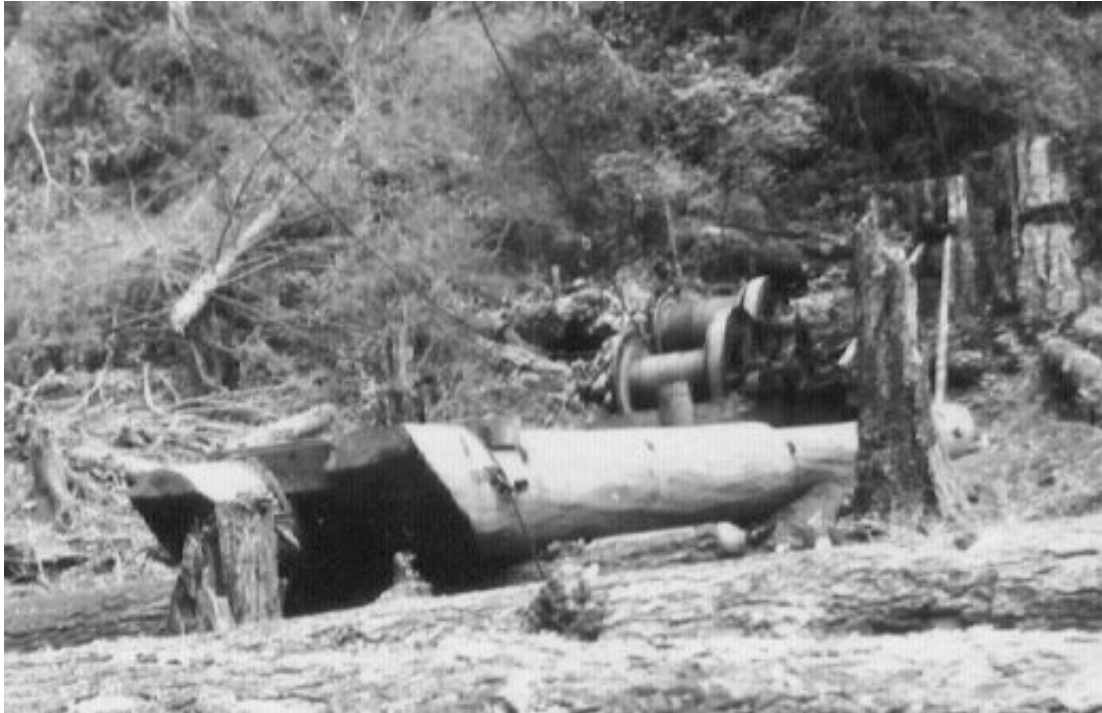
The Willamette 9 by 10 yarder with its 85 HP Ford V8 engine and the new sled Dad and Bud Huff built for it above the falls.
