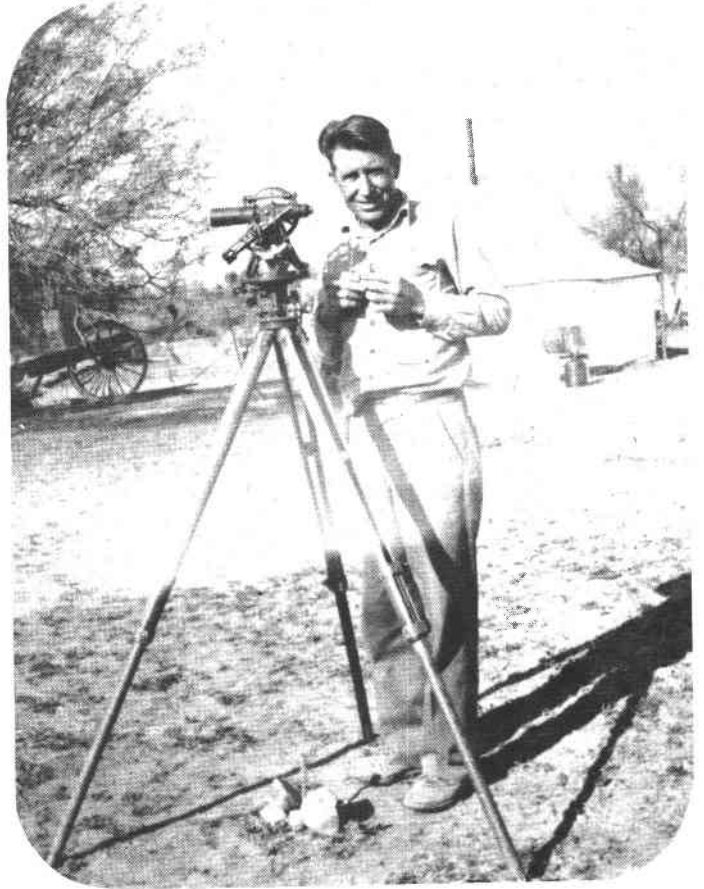
Elliott Pearson at camp at Gila Bend, Arizona, 1947. The instrument is a Hellgate model Gurley transit.
