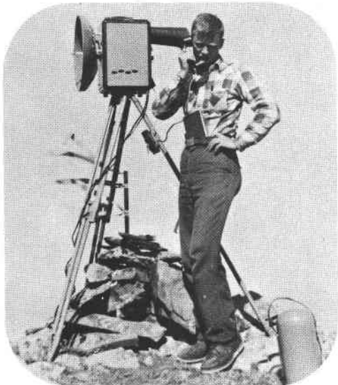
Modern-day (1960) surveying methods: Jerry Harris on a tellurometer station on a point above Minto Flats, Alaska.
